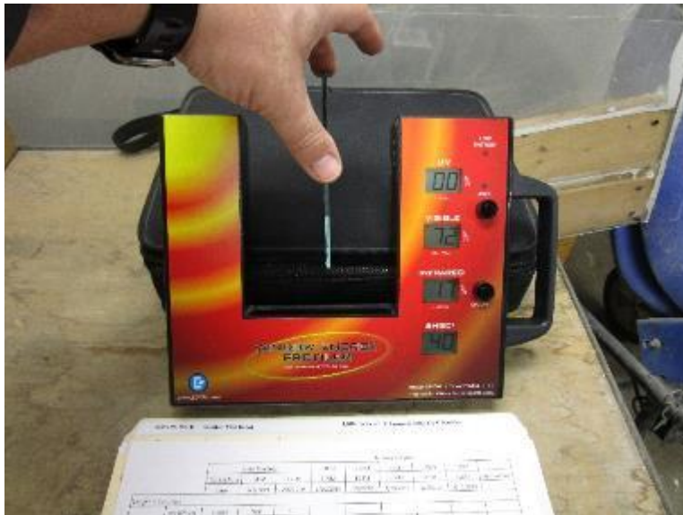
Photo No. 2 EDTM Window Energy Profiler
